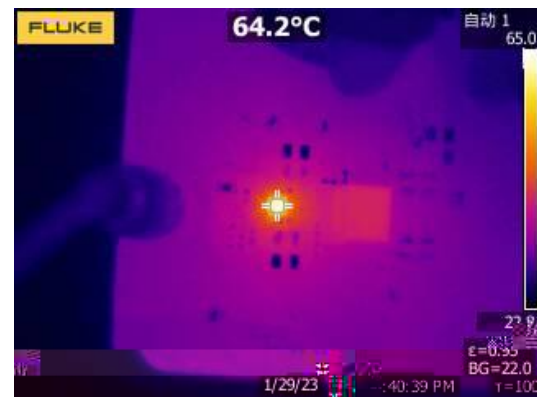
Figure 23. Thermal, 12V IN , 5V OUT , 3A
